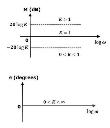
The magnitude plot is a horizontal line, which is independent of frequency. The 0 dB line itself is the magnitude plot when the value of K is one. For the positive values of K, the horizontal line will shift 20logK dB above the 0 dB line. For the negative values of K, the horizontal line will shift 20logK dB below the 0 dB line. The Zero degrees line itself is the phase plot for all the positive values of K.
