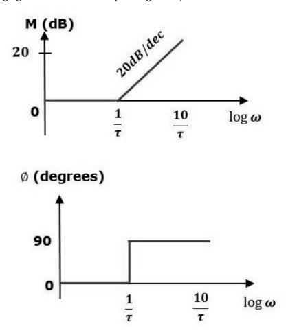
The magnitude plot is having magnitude of 0 dB upto  $\omega = 1\tau \omega = 1\tau$  rad/sec. From  $\omega = 1\tau$  rad/sec, it is having a slope of 20 dB/dec. In this case, the phase plot is having phase angle of 0 degrees up to  $\omega = 1\tau$  rad/sec and from here, it is having phase angle of 90°. This Bode plot is called the **asymptotic Bode plot**.
