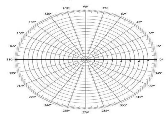
This graph sheet consists of concentric circles and radial lines. The **concentric circles** and the **radial lines** represent the magnitudes and phase angles respectively. These angles are represented by positive values in anti-clock wise direction. Similarly, we can represent angles with negative values in clockwise direction. For example, the angle  $270^{\circ}$  in anti-clock wise direction is equal to the angle  $-90^{\circ}$  in clockwise direction.
