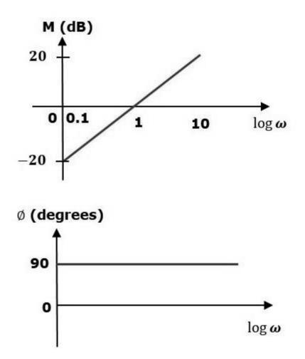
The magnitude plot is a line, which is having a slope of 20 dB/dec. This line started at  $\omega$ =0.1rad/sec having a magnitude of -20 dB and it continues on the same slope. It is touching 0 dB line at  $\omega$ =1 rad/sec. In this case, the phase plot is 90<sup>o</sup> line.
